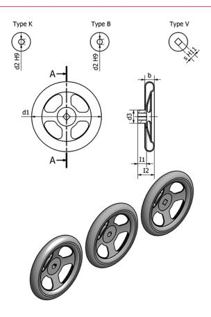
b = 22 d1 = 0 d2 H9 = B14 d3 = 40 I1 = 24 I2 = 44 s H11 = -Spokes no. = 4 Thickness of steel = Thickness of steel = 2.5
